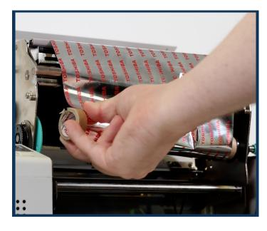
2. Slide the bottom cardbaord core to the right and lift to remove. Remove the top waste ribbon by sliding to the right.
