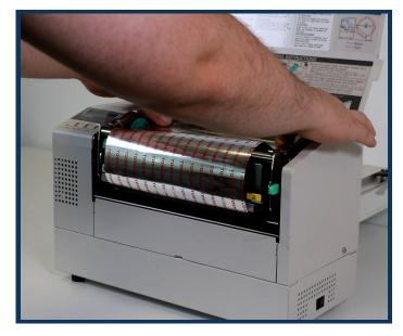
3. Reinsert the cardboard core in the top ribbon slot. Insert your new ribbon to the bottom ribbon slot.
