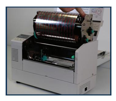
1. The silver foil indicates the end of the ribbon. Open the printer lid and push the green clip to lift the ribbon carriage.
