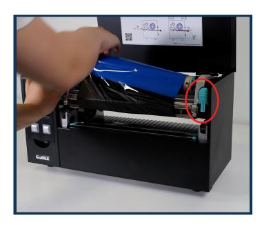
1. Open the printer lid and push the green clips in to lift the ribbon carriage. Remove the ribbon by pushing to the right and lifting up.
