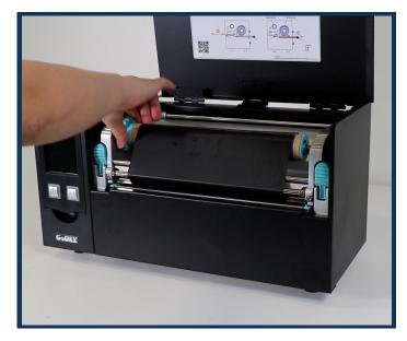
3. Allow a moment for it to dry. Then, resinsert the ribbon and roll to ensure this runs tight and lower the printer lid.
