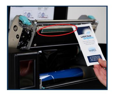
2. Take a cleaning wipe or isopropanol alcohol. Locate the printhead and scrub with the cleaning wipes.
