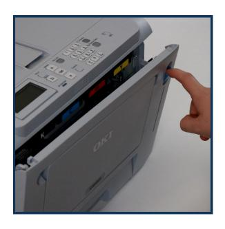
1. Lower the printer lid by pulling the blue tab on the right hand side.
