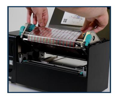
3. Load the new ribbon to the underside of the carriage.
