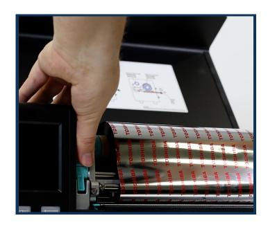
1. Push the green clips in and lift the ribbon carriage up. Pull the excess ribbon off the cardboard core.
