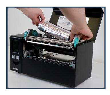
2. Remove the waste ribbon roll by pushing right and lifting. Using the same motion, move the cardboard core to the top slot.
