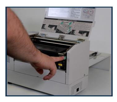
1. Open the printer lid and push the green clips to lift the ribbon carriage. Remove the ribbon by sliding to the right and lifting up.
