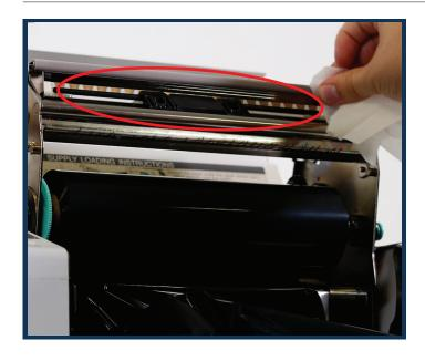
3. Locate the printhead and scrub with the cleaning wipes. Allow a moment for it to dry.
