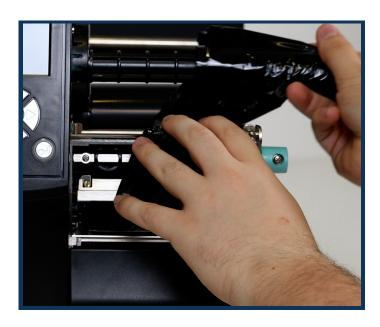
1. Open the printer lid lift the printhead by pulling the green lever up. Then remove the ribbon.
