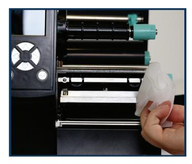
3. Locate the printhead and scrub with the cleaning wipes. Then allow a moment for it to dry.
