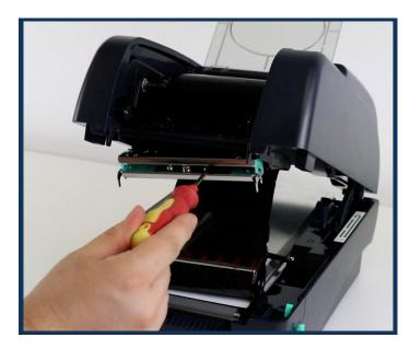
2. Use a screwdriver and slowly push down in the gap as shown to loosen the printhead.
