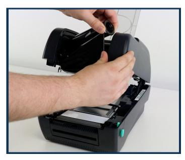
1. Turn off the printer and open the printer lid. Remove the ribbon by pushing it to the left and lifting up.
