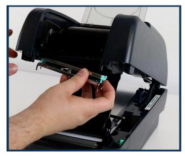
4. Push the printhead into place one side at a time until it clicks in place. Reinsert the ribbon.
