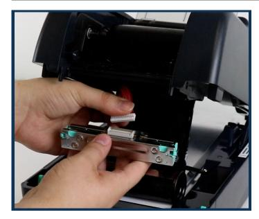
3. Detach the cable at the back of the printhead. Take your new printhead and plug in as shown.
