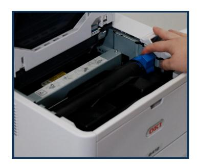
2. To replace the toner, pull the lever towards you, on the toner. and lift from the right side. Replace with the new toner.
