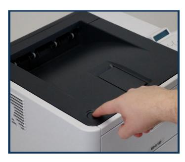
1. Turn off the printer and lift the lid by pressing the button as shown.
