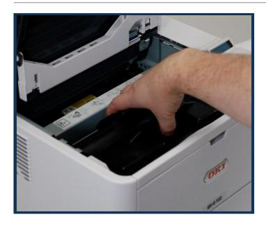
3. To replace the image drum, lift the image drum out as shown and replace with a new image drum by slowly dropping it in. Then replace the toner with an old or new one, which can be found in the 'replace toner' guide.
