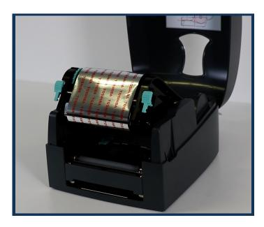
1. The silver foil indicates the end of the ribbon. Open the printer lid and push the green clips to lift the ribbon carriage. Remove the waste ribbon on top by sliding to the left.
