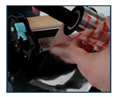
2. Remove the black plastic core from the waste roll and reinsert into the new ribbon. Move the empty cardboard core to the top.
