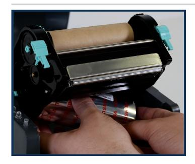
3. Insert the new ribbon to the back slot and ensure the loose roll is face down.
