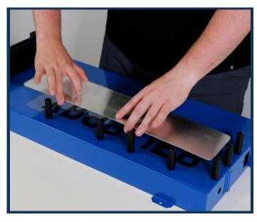
1. Print the registration onto your clear film. Peel back the adhesive cover on the aluminium and align over the film media.
