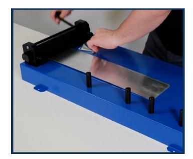
2. Ensure the exposed adhesive is on the side nearest the roller. Roll through the number plate laminator roller.
