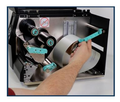
2. Lift the green lever and remove the used reflective roll. Replace with a new roll and lower the green lever.
