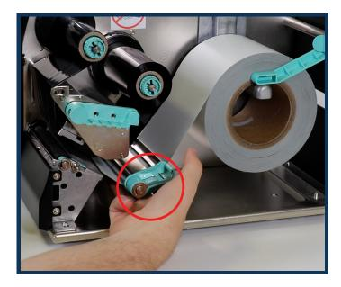
3. Pull out the green clip towards you. Feed the reflective up and under to where the printhead sits.
