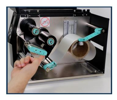
1. Open the lid of the printer. Lift the green clip at the front of the printer to lift the printhead. Roll the reflective back.
