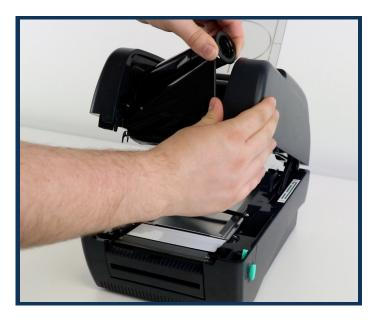
1. Open the printer lid and remove the ribbon by pushing to the left and lifting up.
