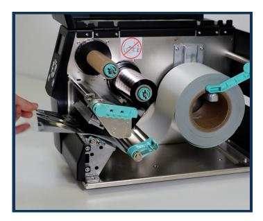
3. Insert the new ribbon to the back slot and feed the ribbon under the printhead as shown.
