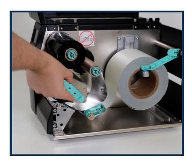
1. The silver foil indicates the end of the ribbon. Open the printer lid and push up the green lever to lift the printhead.
