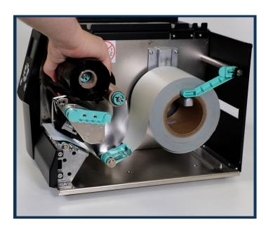
2. Slide the waste ribbon off and pull free from the cardboard core. Move the cardboard core to the front ribbon slot.
