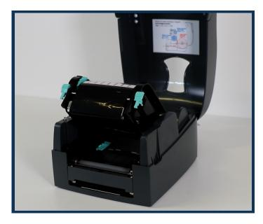
1. Open the printer lid and push the green clips to lift the ribbon carriage. Remove the back waste ribbon by sliding to the left.
