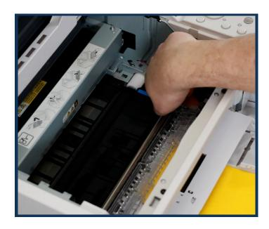
2. At the bottom of the printer, lift the clear panel as shown.
