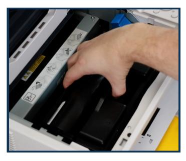
1. Open the printer lid by pushing the bottom left button and remove the image drum as shown.
