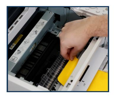
3. You can now pull out the jammed reflective media. Load up the reflective for printing.
