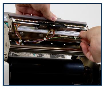
3. Take the new printhead and plug in the three cables. Reinsert the printhead back into place, sliding in from right to left.
