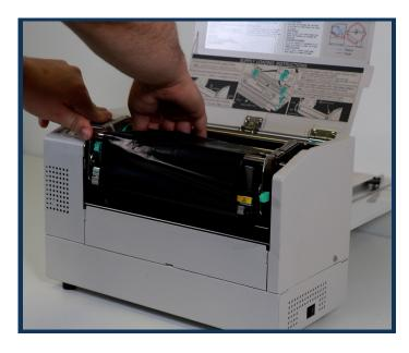
1. Open the printer lid and push the clip down on the right side of the printer. Remove the waste ribbon by sliding it to the right.
