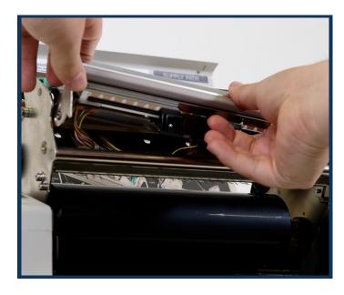
2. Slide the bracket to the right where the printehead is and gently pull it away. Carefully unplug the three cables.
