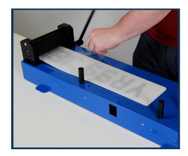
2. Peel back the adhesive cover on the acrylic and align to the pegs, placing over the reflective. Roll through the laminator roller.
