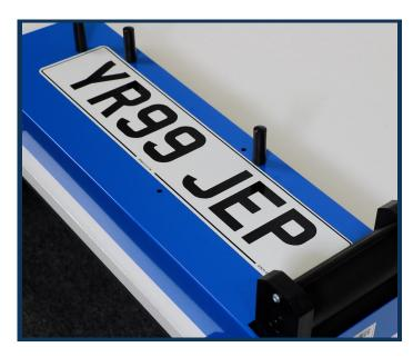
1. Print your number plate and align your reflective to the pegs on the number plate laminator.
