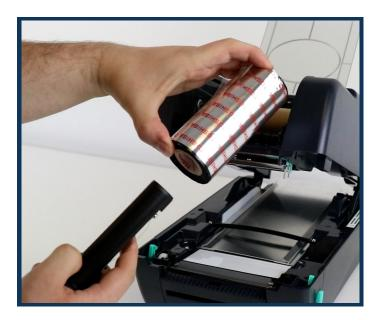
2. Remove the black plastic core from the waste roll and reinsert into the new ribbon. Move the empty cardboard core to the front.
