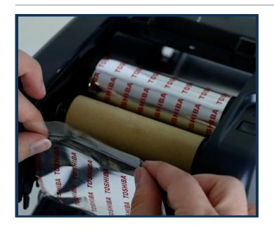
3. Insert the new ribbon to the back ribbon slot and ensure the loose roll is face down.
