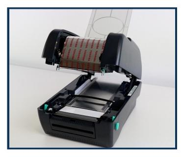
1. The silver foil indicates the end of the ribbon. Open the printer lid and remove the ribbon by pushing to the left and lifting up.
