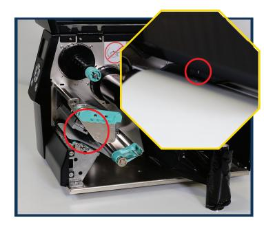
2. The sensor is the white mark as shown. Roll out the reflective until the perforation aligns with the white marker.
