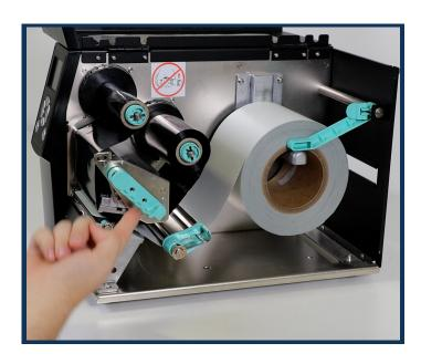
1. Open the printer lid and lift the green lever up to lift the printhead. Roll the ribbon to ensure it runs tight.
