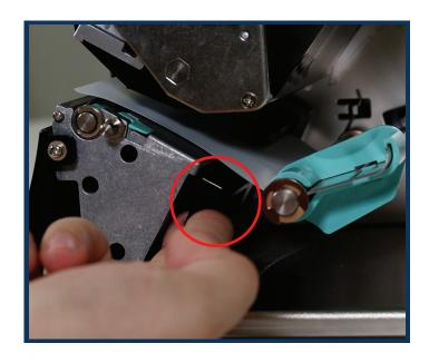
3. Pull the lever as shown - your printer is now aligned to the roll.
