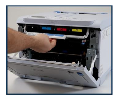
2. Pull out the tab L2, then lift to lift the lid of the printer. Now pull out the image drum drawer.
