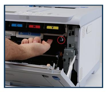
1. Pull the tab down to open the printer. To access the image drum, pull out the tab labelled L1 (circled).
