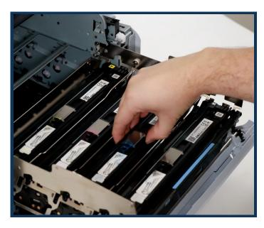
3. Lift out the corresponding image drum out of the drawer and replace with a new one. Then, push the drawer back in until it clicks into place, lift the lid down and ensure L2 and L1 are pushed back in. You can begin printing again.
