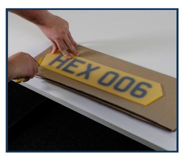
3. On a cutting mat, use a craft knife to cut off the excess reflective. Peel off the protective film. You're now ready to use your hex number plate.
