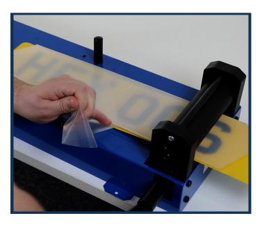
2. Run the Number plate through the roller on your number plate laminator. Ensure this is on the 'acrylic' setting.
