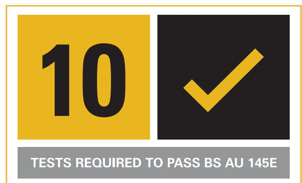
*\*The full range of tests includes; colorimetric, retroreflection, resistance to bending, resistance to solvents, thermal resistance, resistance to impact, resistance to abrasion, resistance to corrosion, resistance to weathering and opacity of the characters in near infrared.*
